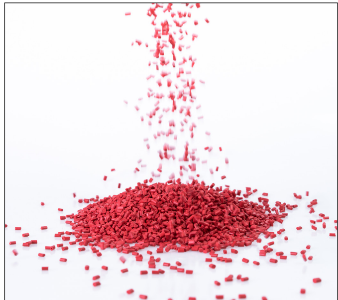
Fig. 2: Plastic granulate for injection molding or extrusion
