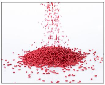
Fig. 2: Plastic granulate for injection molding or extrusion
