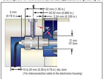
Figure 7. Cylinder end cap mounting detail reference
