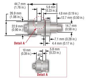
Figure 8. Pressure fit rod style 'S' details
