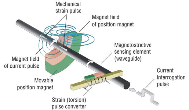
Fig. 1: Time-based magnetostrictive position sensing principle
