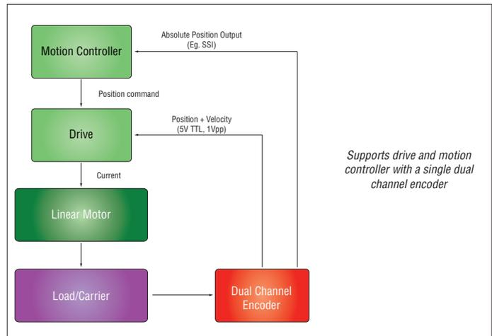
Fig. 3: Dual Channel Encoder
