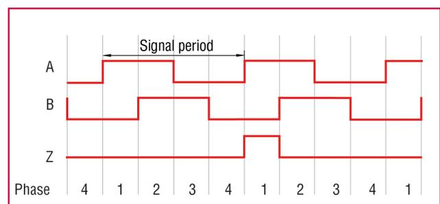
Fig. 2: Gated to Leading Signal Edge
