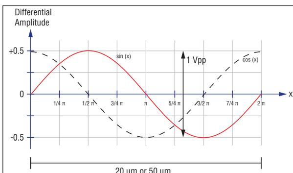
Fig. 1: Differential Amplitude and Signal Period
