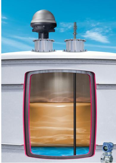
Radar is available as either 'through the air' radar or guided wave radar. The difference between the two types of radar is the 'through the air' radar sends the microwaves focused by an antenna through the air to determine the liquid level whereas the guided wave radar sends the microwaves through a pipe or metal braid to help guide the path of the microwaves.
