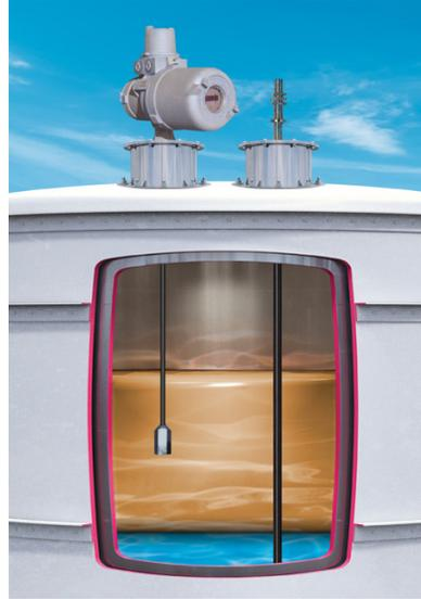
mounting requirements for the different level technologies are dependent on the structure of an existing tank and can require no or several tank modifications. Selecting the level technology that best fits the tank can save thousands of dollars in installed costs. The costs of tank modifications can be broken down into the costs for tank openings and the cost for stilling wells. The costs of tank modifications increase with every additional opening requirement for the tank.
