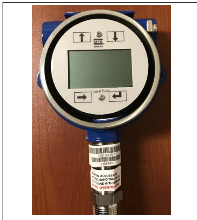
Fig. 1: Housing without cover
