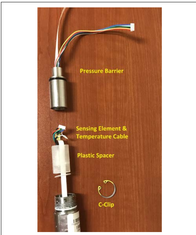
Fig. 11: Explosion proof cartridge
