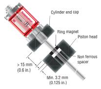
Figure 6. Model RH rod-style mounting
