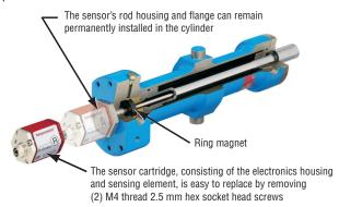
Figure 7. Fluid cylinder installation
