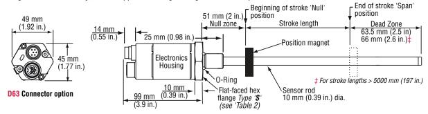
**Figure 7.** Model RH Rod-style sensor dimension reference (shown with **D63** connector option)
