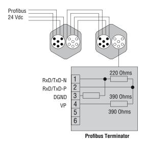
For (D53) connection types, a separate 4-pin connector and cable is used for the supply voltage.
