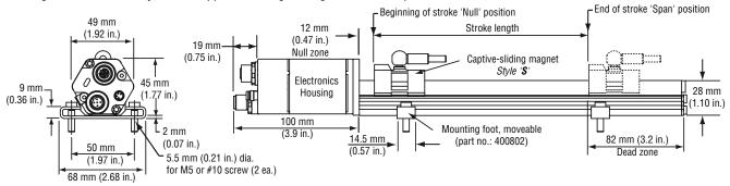
Figure 4. R-Series Model RP Profile-style sensor dimension reference (Shown with the D53 connector option)
