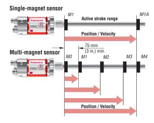
Figure 2. Single and multi-magnet output diagram
