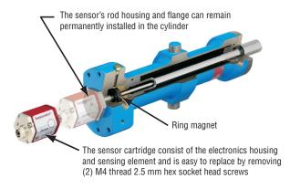
Figure 11. Fluid cylinder installation
