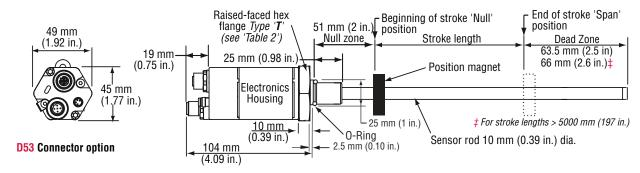
**Figure 8.** Model RH Rod-style sensor dimension reference (shown with **D53** connector option)
