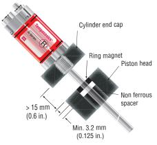
Figure 10. Model RH rod-style mounting
